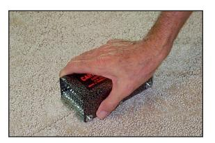
These amazing tools can obscure carpet seams—even badly cut seams—with much less time and effort than any other method. Carpet Tractors can also improve the appearance of poor seams caused by numerous other installation problems.
